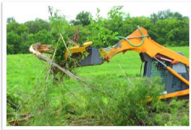
Figure 12: Skid steer with tree pulling attachment
