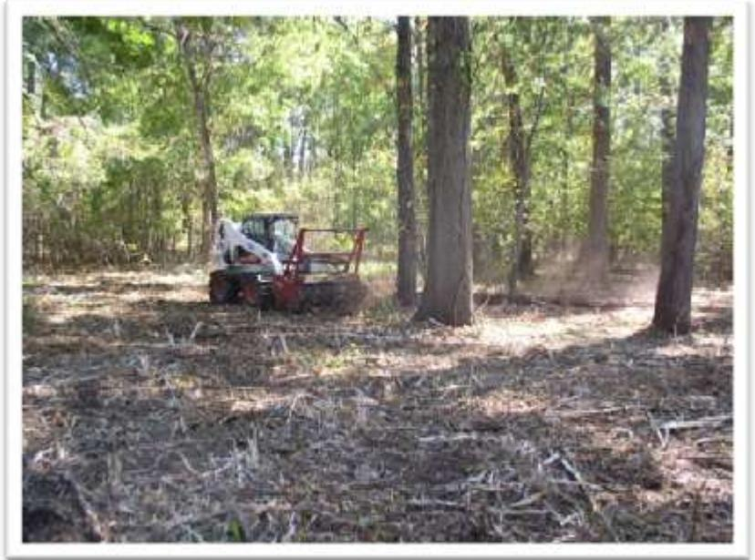
Figure 13: Heavy duty brush cutter shredding bush honeysuckle
